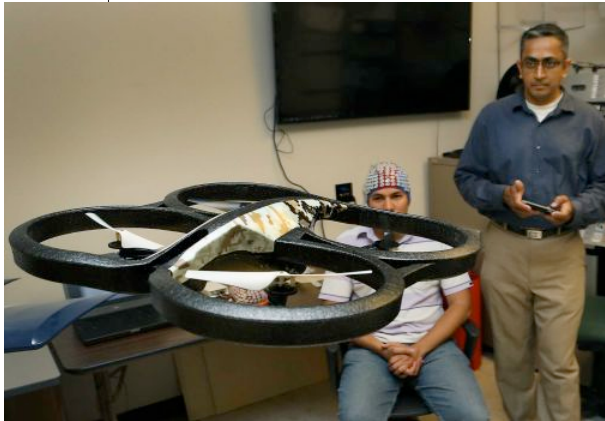
Figure 7. A helicopter controlled by brain waves.
