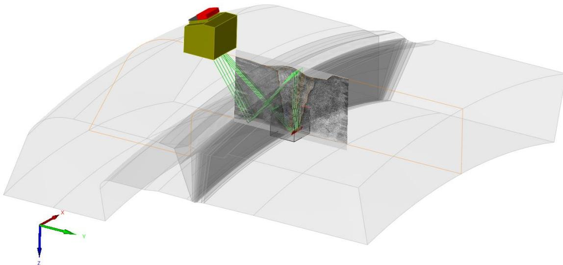
**Figure 2.** Simulation of dissimilar metal weld examination [8]
