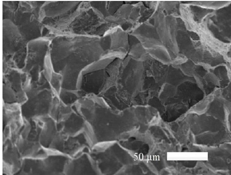
**Figure 3.** Cleavage fracture on irradiated Russian RPV steel (SEM)
