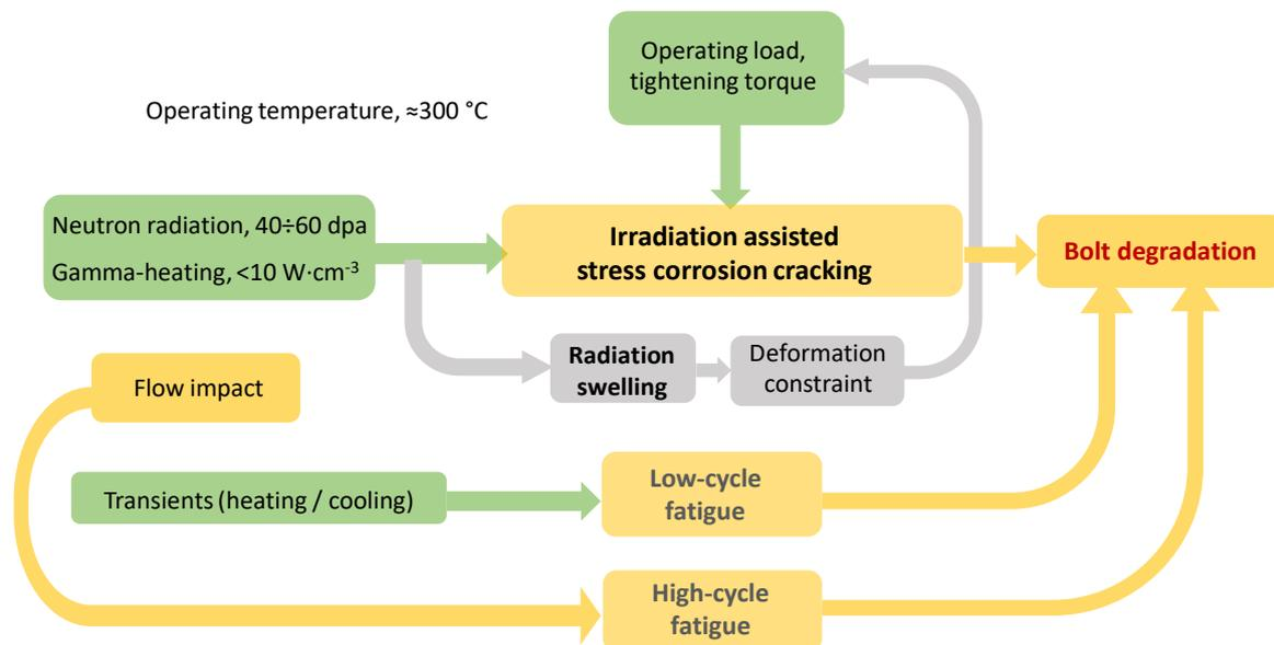
**Figure 4.** Loading of and their impact on baffle bolts [13]
