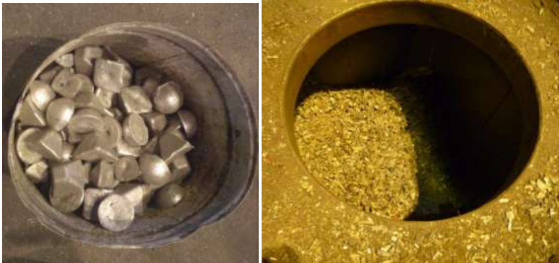
Figure 1. “Mokka” (left) and “shredder” (right) deoxidizing aluminium
